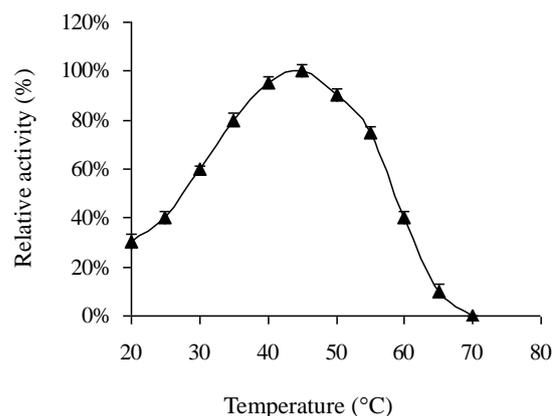
**Figure 5.** Dependence of lytic activity on temperature for rSLZ. The rSLZ activity assay was measured against *Micrococcus lysodeikticus* in 66 mM potassium phosphate buffer, pH 6.24, at different temperature (20°C to 70°C) after incubation for 30 min. Recombinant SLZ activity measured at 45°C represented 100% activity. The experiment for each group was done in duplicates and the error was always below 5%.
