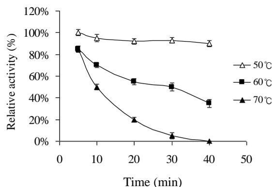
**Figure 6.** Thermostability of purified rSLZ at 50°C, 60°C, and 70°C. The rSLZ activity assay was measured against *Micrococcus lysodeikticus* in 66 mM potassium phosphate buffer, pH 6.24, at 25°C after incubation for different times at 50°C, 60°C, and 70°C. The experiment for each group was done in duplicates and the error was always below 5%.
