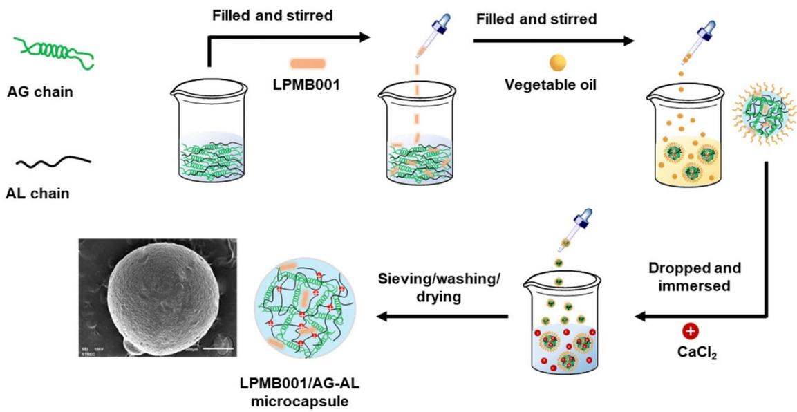
**Figure S2.** Schematic for steps of preparation of LPMB001/AG-AL.
